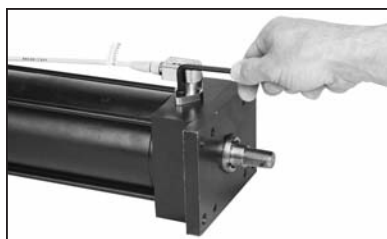
Bolt sensor to cylinder.
